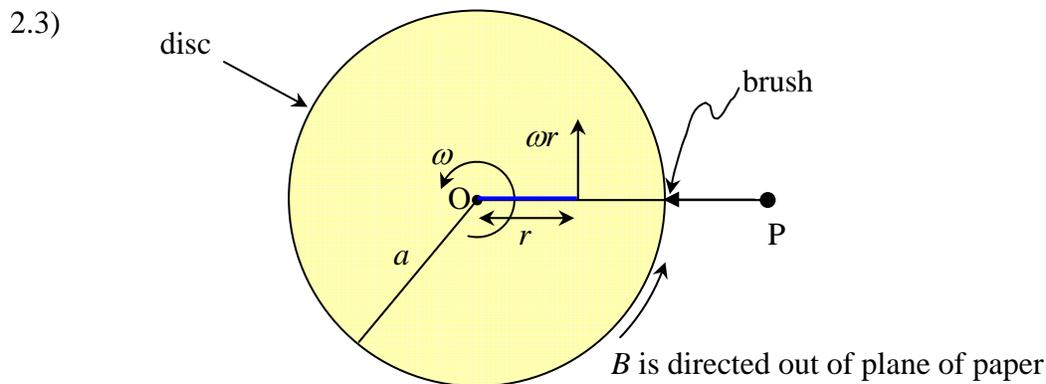
The electric field intensity ( $E$ ) at distance  $r$  from the centre of the axle is
