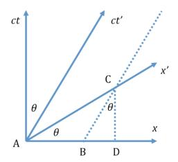
The stick is represented by the segment AC. The length AC is equal to  $\sqrt{\frac{1+\beta^2}{1-\beta^2}}L$  in the S frame. The stick length in the S frame is represented by the line AB.
