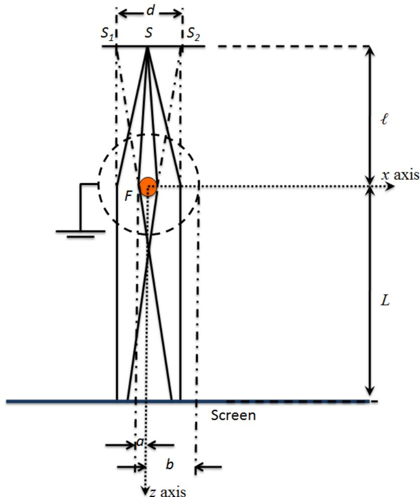
The electron “biprism” consists of a grounded cylindrical wire mesh with a fine filament  $F$  at the center. The distance between the source and the “biprism” is  $l$ , and the distance between the “biprism” and the screen is  $L$ .
