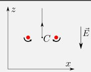
Electric force upon the loop  $F=-2\pi ER_0|\lambda|$  is constant and fluid momentum linearly depends on time
