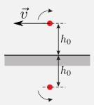
Illustration of the image method for the straight vortex filament near a flat wall
