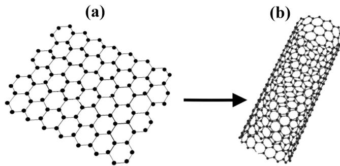
**Figure 3.** Graphene (a) and carbon nanotube (b).
