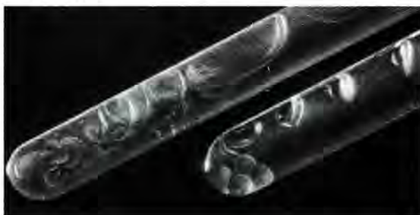
Figure 4. The process of boiling proceeds quite differently in test tubes with distilled and tap water.
