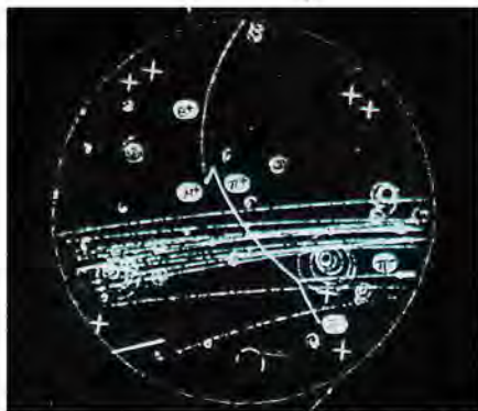
Figure 3. A photograph of processes of interaction and conversion of elementary particles in a liquid-hydrogen bubble chamber.
